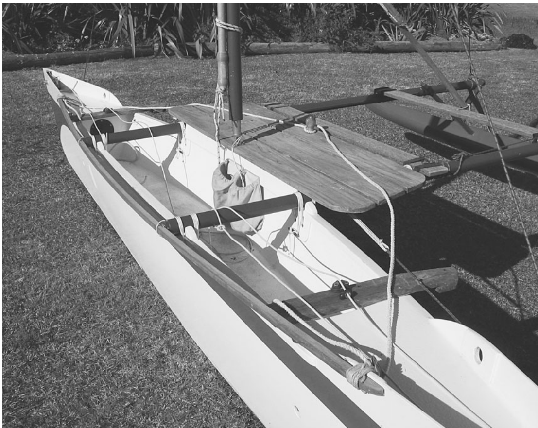
FIGURE 10-20. A windward-side hiking seat on the T2, with a wooden knob bolted in place to snub the sheet. Note the leeward-side guide rail to aid in shunting an Oceanic lateen sail.
