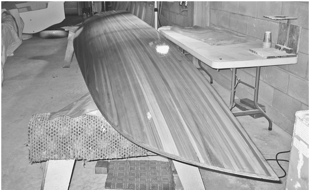
FIGURE 6-21. Clay Ghylin's planked and glassed T2 hull. (Photo courtesy Clay Ghylin)
