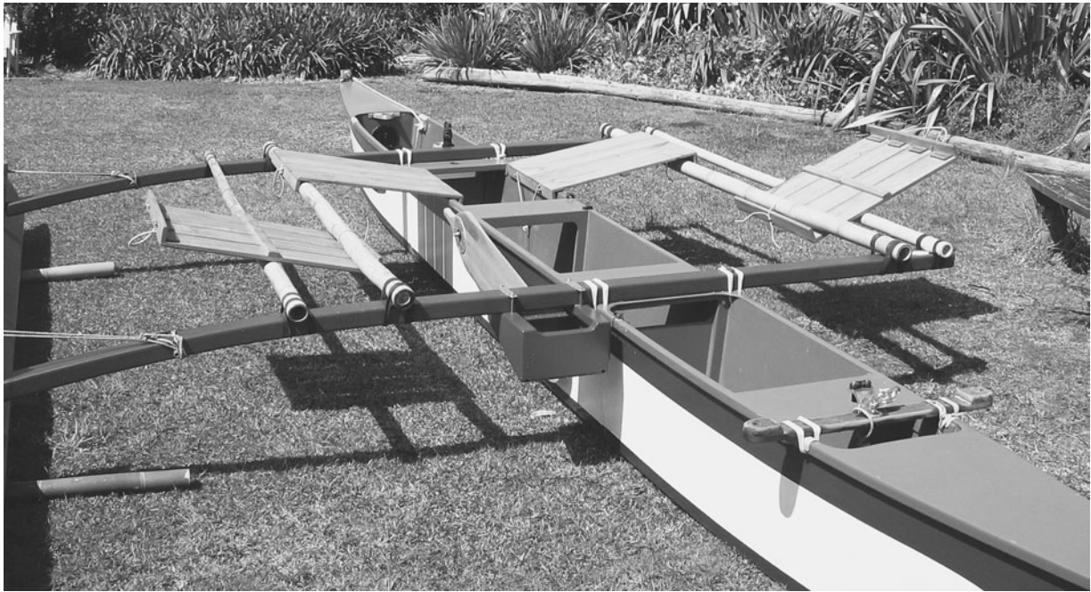
FIGURE 10-19. The hiking seats on the Wa'apa pivot outboard for paddling and rest against a second bamboo pole.
