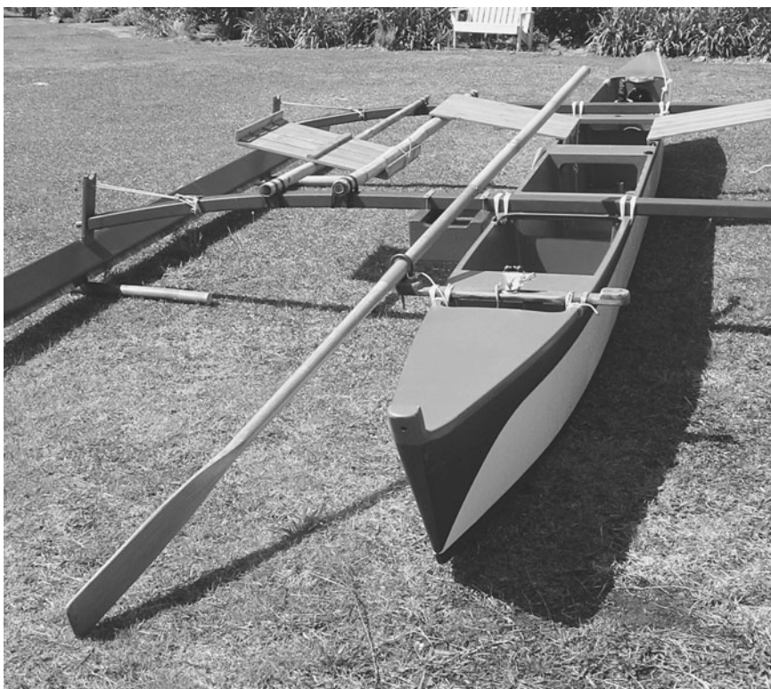
FIGURE 10-3. A steering oar in position and pivoting on a hardwood spreader lashed to the gunwales. The lashing holes, which are securing the steering bracket, are those used for the cross beams when the hull is in the 16' (4.8m) configuration.
