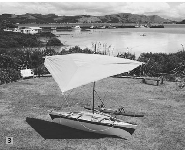
FIGURE 12-13. The forward tack line is released while the aft tack line is taken in, allowing the yard to pivot to a horizontal position. A light tension is kept on the tack line at both ends of the yard to avoid oscillation.
