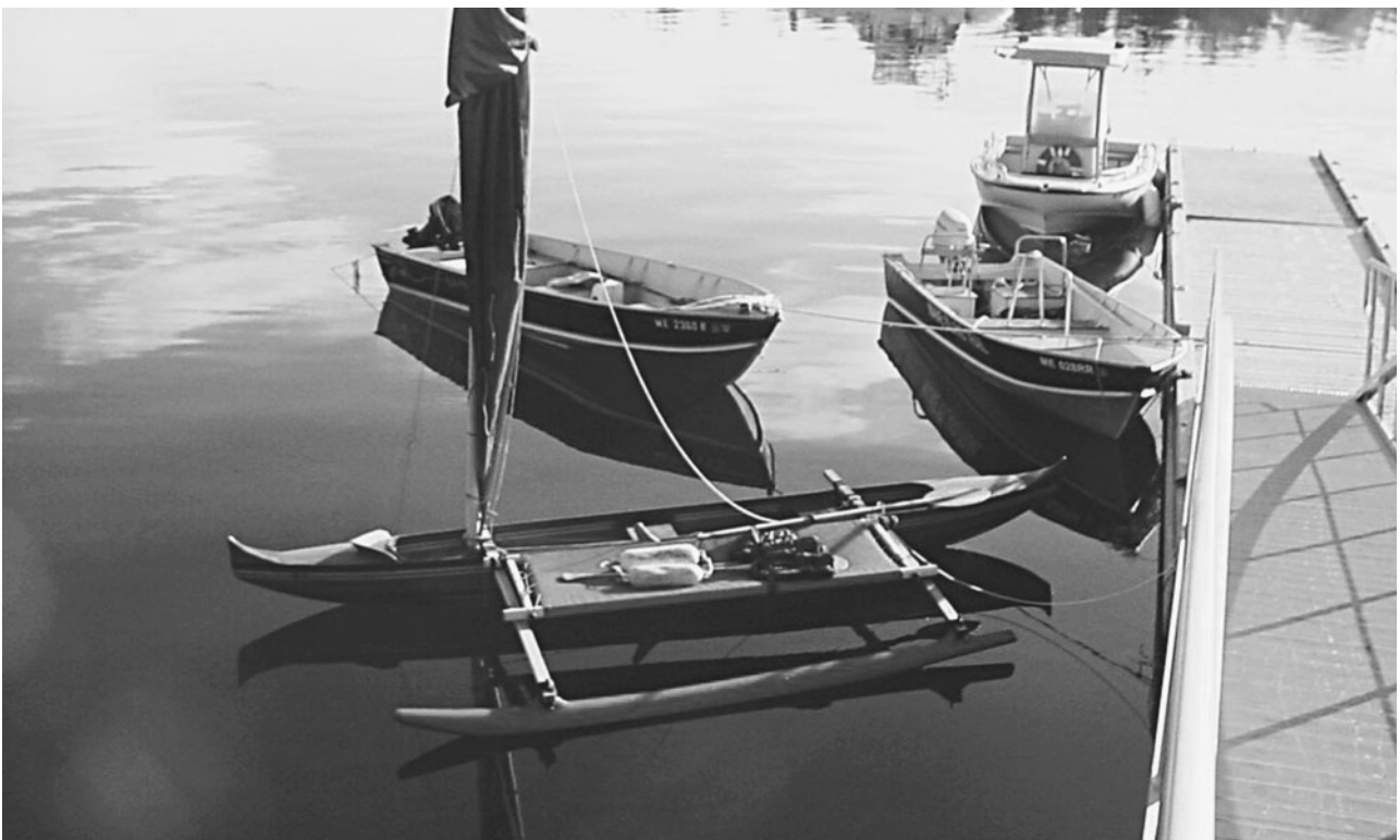
FIGURE 1-12. Michael Wise's Ulua equipped with a fabric trampoline. (Photo courtesy Michael Wise)
