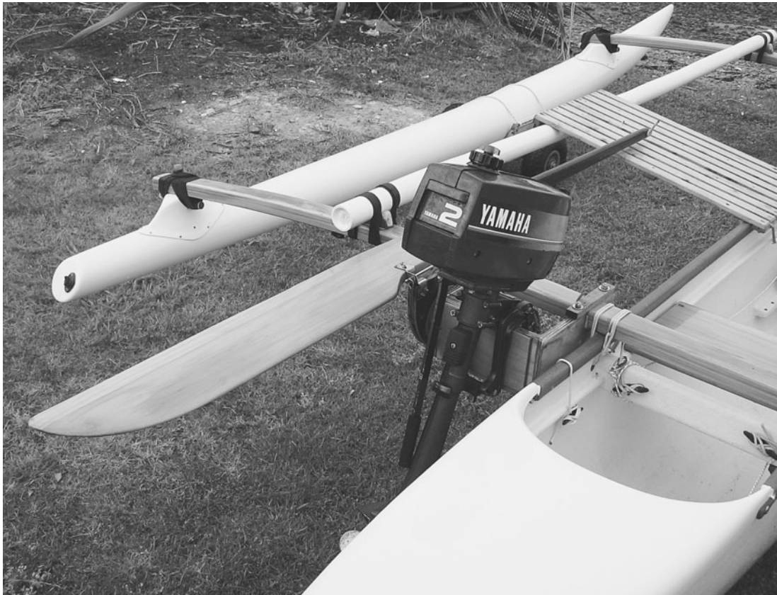
FIGURE 10-18. A kick-up rudder and outboard motor mounted on the Ulu'a's bracket. Note the anti-torque line coming from the bottom of the bracket, over the gunwale, and tied to a cleat.
