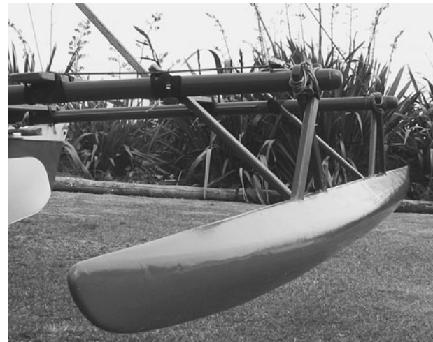
FIGURE 8-24. Tarawa's original foam-filled ama has an inverted "V" plywood deck.
