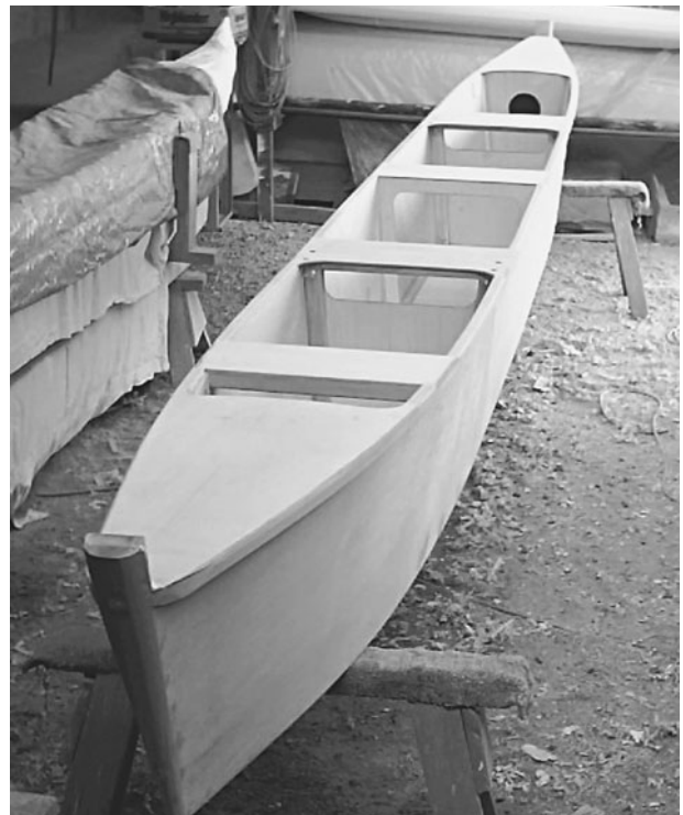
FIGURE 7-13. Three hull sections bolted together, complete with foredecks and seats.
