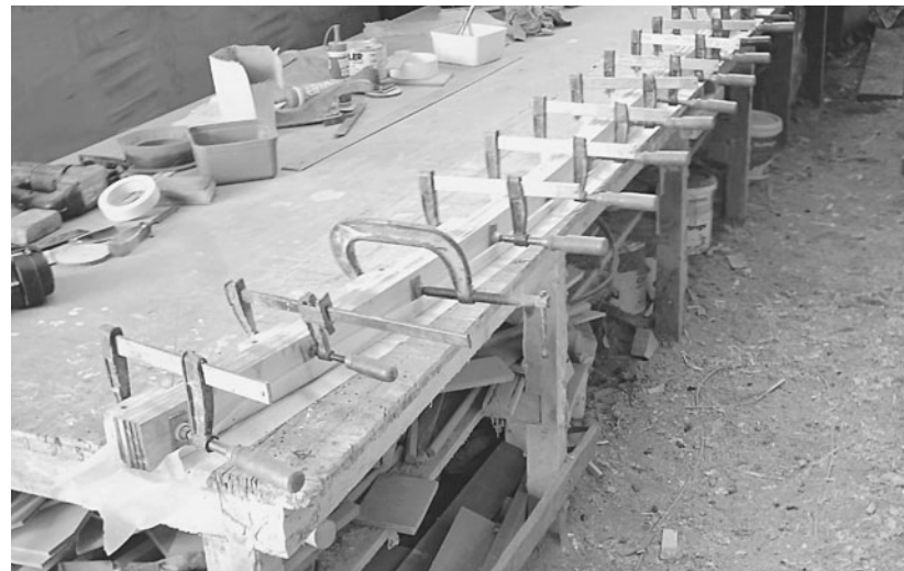
FIGURE 9-14. (ABOVE LEFT) A laminating jig for solid iakos consists of a row of wooden blocks screwed to a flat surface. Note the waxed paper taped in place to prevent gluing the beam to the table or the blocks.
