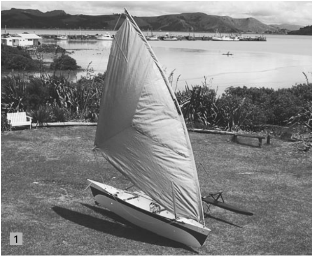
FIGURE 12-11. Gibbons/Dierking rig close-hauled on a port tack.
