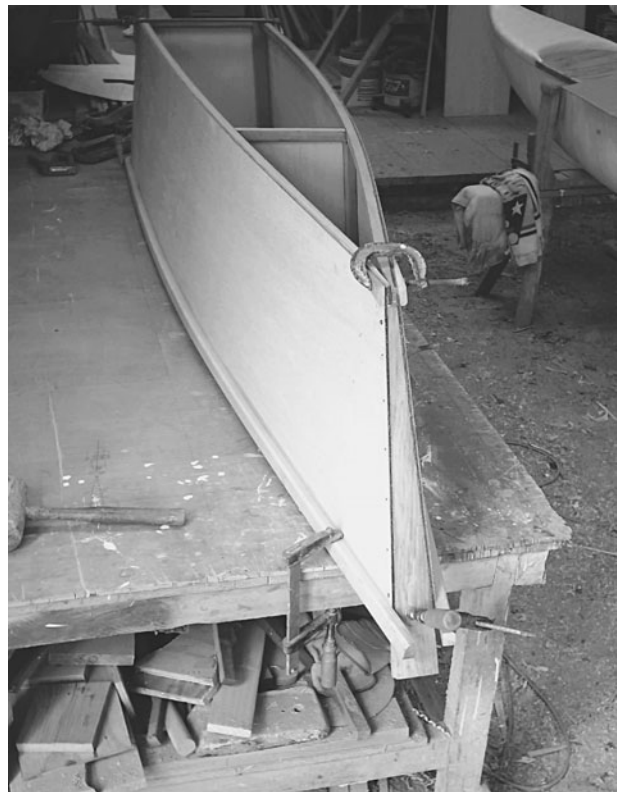
FIGURE 7-10. Side panels are fastened to the bulkheads and bent together at the stem.
