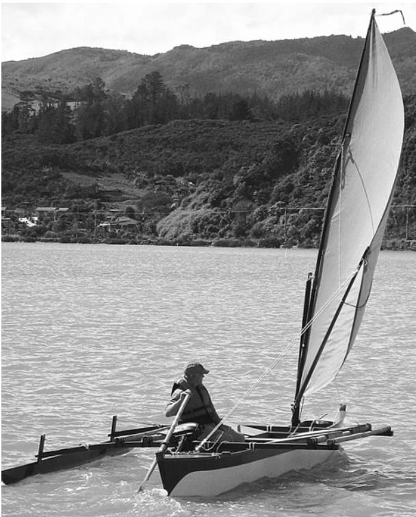
FIGURE 3-13. (ABOVE LEFT) 24' (7.2m) Wa'apa with tacking rig. (Photo courtesy Rose Turner)
