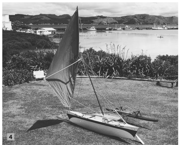
FIGURE 12-14. The tack of the sail is pulled down to the new bow, and the tack line is secured in a cam cleat.
