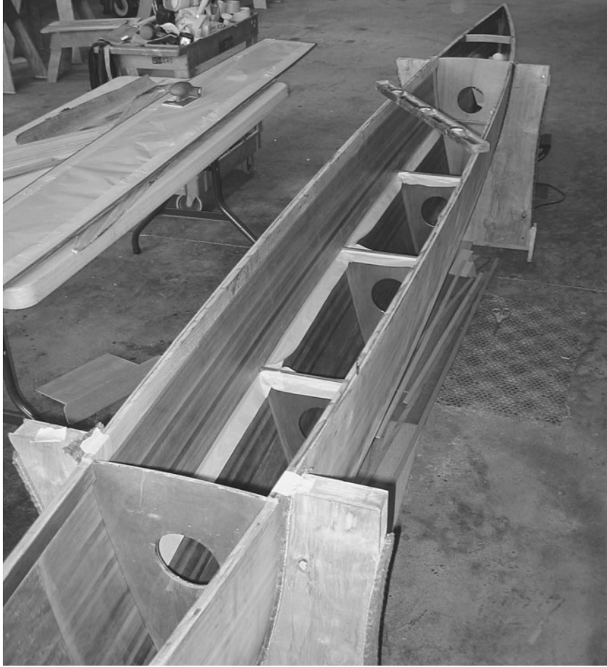
FIGURE 6-22. T2 bulkheads and cockpit floor support structure in place. (Photo courtesy Clay Ghylin)
