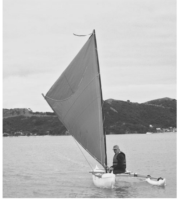
FIGURE 1-7. (ABOVE LEFT) Ulua sailing on a starboard tack, with the ama to leeward and the sailor seated in the hull. (Photo courtesy Rose Turner)
