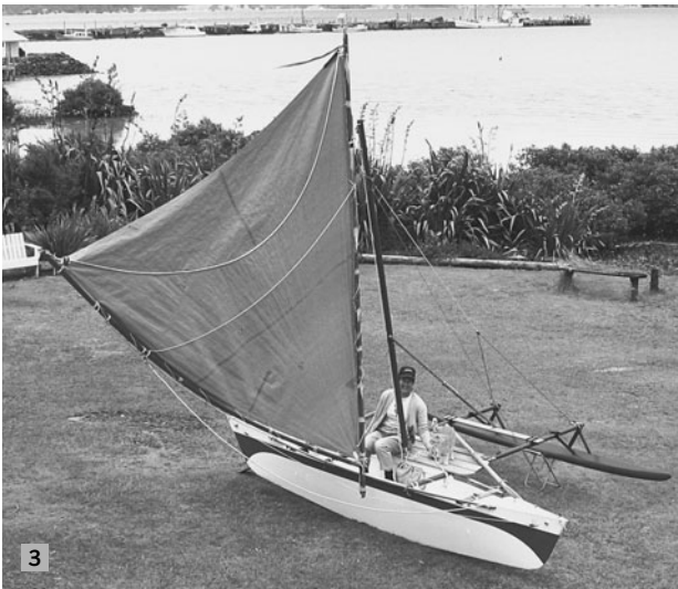
FIGURE 12-8. The tack line is used to pull the yard along the leeward side of the hull.
