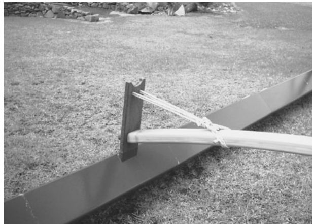
FIGURE 8-25. The Wa'apa connection method allows limited movement of the ama in the pitch axis.
