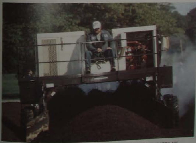
A professional turns his compost to aerate it. Photograph by Ken Hammond, USDA-ARS.
