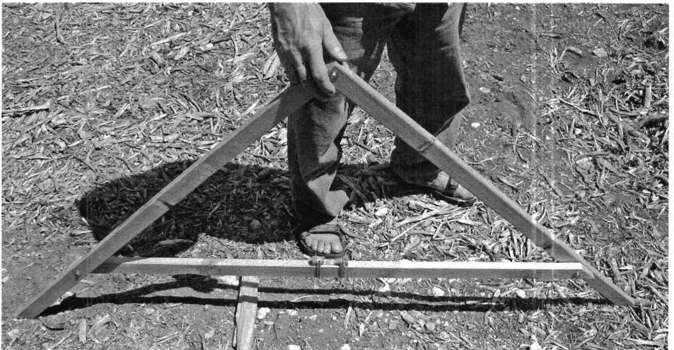
Fig. A2.14. Chris Meuli's line-level A-frame. A bubble level tool is lashed to horizontal bar below Chris' toes. Chris bolts his A-frame together with wing nuts so he can disassemble and fold it up for easy storage. His A-frame is only as tall as his waist, which allows him to use the tool under the branches of trees.
