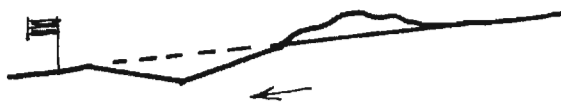
Fig. 9.22C. Drain with basin dug upslope of flagging and dirt cast upslope of basin to form berm. Final drain size 11 inches (30 cm) deep, 16 feet (4.8 m) wide.
