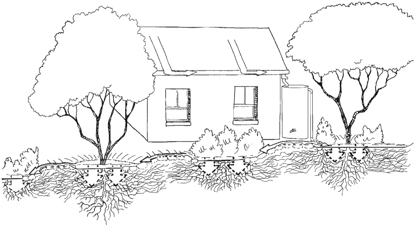
Fig. 1.15. Downspout directing water to a high point at the site to passively spread and infiltrate water over more of the site. Water from cistern faucet and overflow pipe is gravity-distributed to all areas downslope. Note: Terraced basins are at least 10 feet (3 m) from building foundation.
