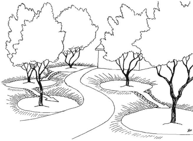
Fig. 5.5. Terraced or stepped basins from which overflow water will flow down a stabilized spillway to the next basin below. The bottom of each basin is lower than the height of its spillway so water infiltrates throughout the landscape—each stepped basin of the way.
