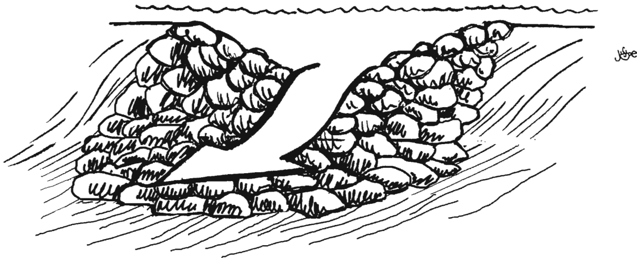
Fig. 5.16. Spillway with stone stabilization. The center must be the low point with raised banks similarly stabilized with stone so the water does not cut a new, more-erosive path. The bottom of the slope where the soil becomes level is also stabilized to calm the faster-moving water that flows down the slope.
