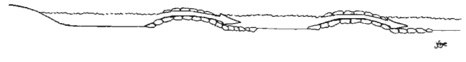
Fig. 5.15B. Stabilized spillways connecting basins on a flat site. Basin depths are the same here, though they can vary randomly. Spillway elevations on such flat sites can all be the same, whatever the basin depth.
