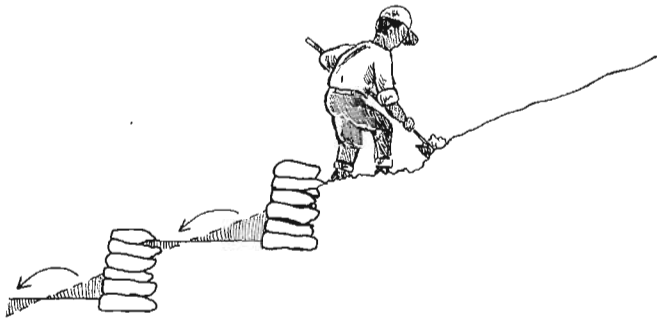
Fig. 3.11. Building terraces starting at the bottom of the slope and working up
