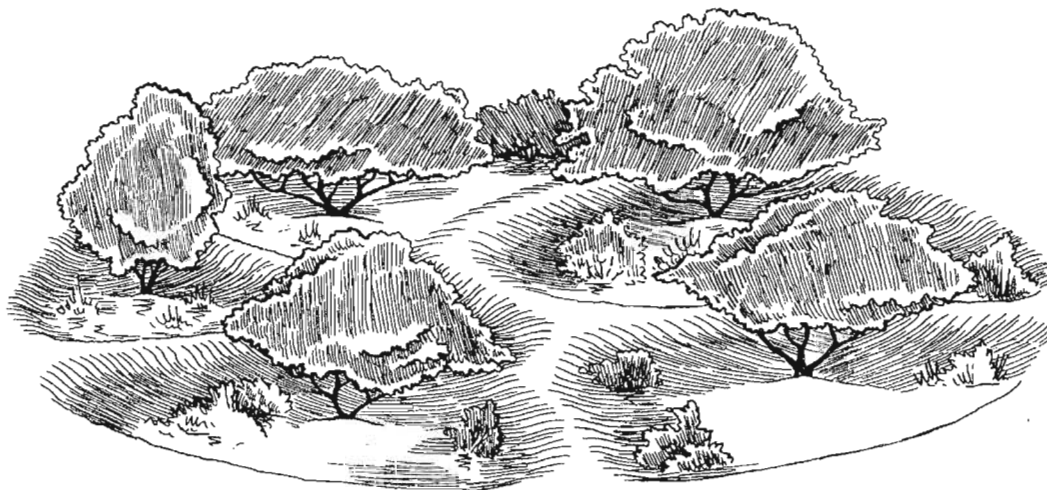
Fig. 5.8. Large basin divided into smaller basins
