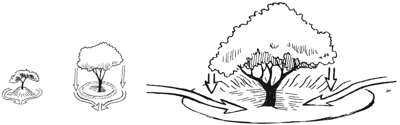
Fig. 5.3. From left to right, a tree planted atop a mound from which water and soil drain away; within a circular berm which diverts area runoff and any leaf drop falling outside the berm away from the tree; and within an infiltration basin toward which the surrounding area is sloped so all direct rainfall, surrounding runoff, and leaf drop is harvested. These trees could've all been the same size at planting, and planted at the same time, though their current size reflects how the vegetation will respond to the degree to which different landforms drain or harvest resources.
