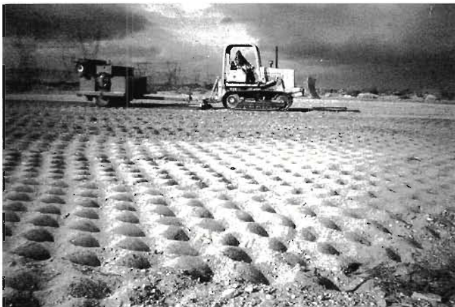
Fig. 6.1. Bulldozer pulling an imprinting roller. Imprints are in the foreground.
