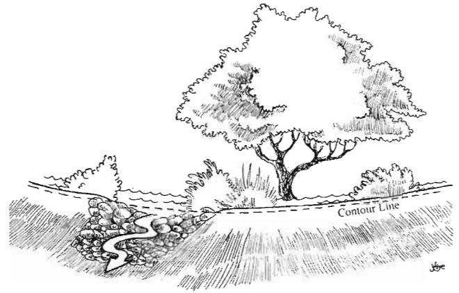
Fig. 2.14B. A successful level berm with a planned, stabilized overflow (above the bottom of the basin) allows surplus water to exit the berm 'n basin, while the majority of the water is harvested within the earthwork.
