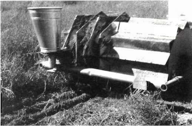
Fig. 6.8. An early style of imprinter squashing tumbleweed so it acts as a mulch for the imprints
