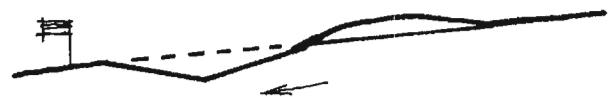
Fig. 9.22D. Completed drain. Uphill berm graded to form road, downhill overflow apron is undisturbed.
