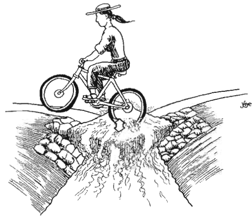
Fig. 10.34B. Spread-out, shallow, and passable flow with check dam. Arrow denotes deepest depth of water. The gabion itself is just downstream of the road, so that the road is on the silted-up terrace behind the gabion, not on the gabion itself.
