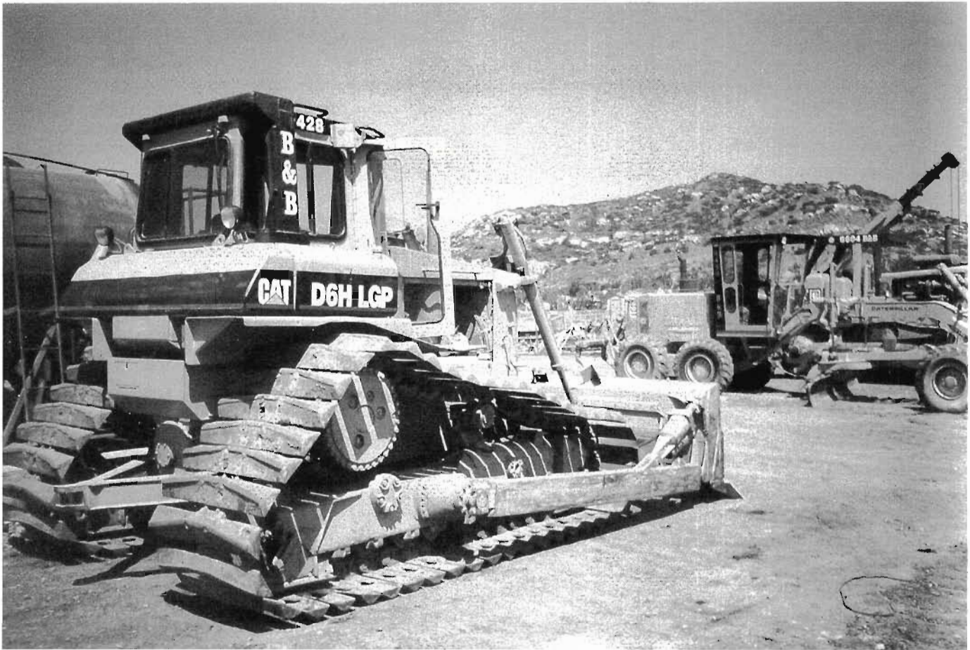
Fig. 6.5. A bulldozer with self-cleaning tracks
