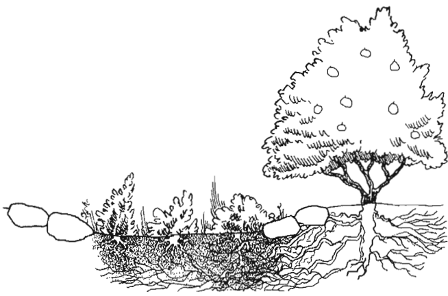
Fig. 11.13. A tree needing better drainage planted beside a basin where its roots can easily tap the harvested water, while leaving the base of the tree (root crown) well drained and dry to reduce the chance of crown rot
