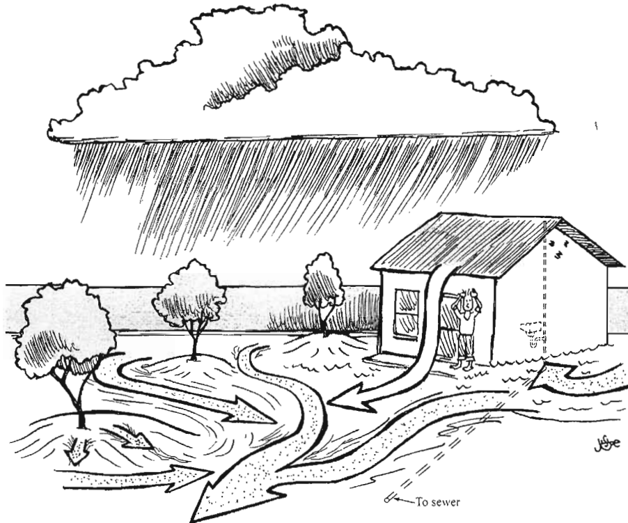
Fig. E.1. The wasteful path to scarcity . The site rapidly dehydrates itself by erosively draining rainwater and runoff away to flood downslope areas and contaminate surface water with sediment. Greywater is lost to the sewer. Costly municipal or well water is pumped in to replace the free water that was drained away. Leaf drop/mulch is also drained away, further depleting fertility and water-holding capacity. This leads to a depletion of resources and feeling scared in the city due to the resulting scarcity .
