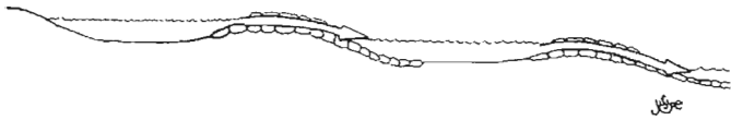
Fig. 5.15A. Stabilized spillways connecting terraced basins on a gentle slope. Note that the bottom of each basin is lower than the top of its spillway so only surplus water overflows the basins, while the majority of the water sticks around and infiltrates. Finished basins are also vegetated and mulched to enhance the infiltration.
