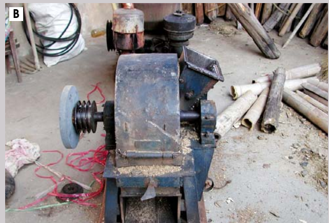
Figure 3. Making sawdust with collected branches A: Collected branches stored in the corner of a farmer's house B: Sawdust making machine
