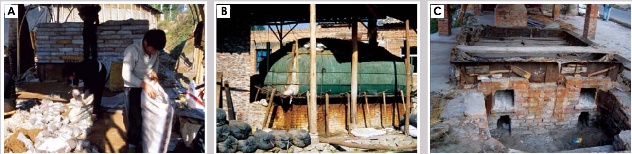
Figure 5. Sterilization kiln A: Arrangement of sacks with bags B: Sterilization with kiln C: The structure of kiln
