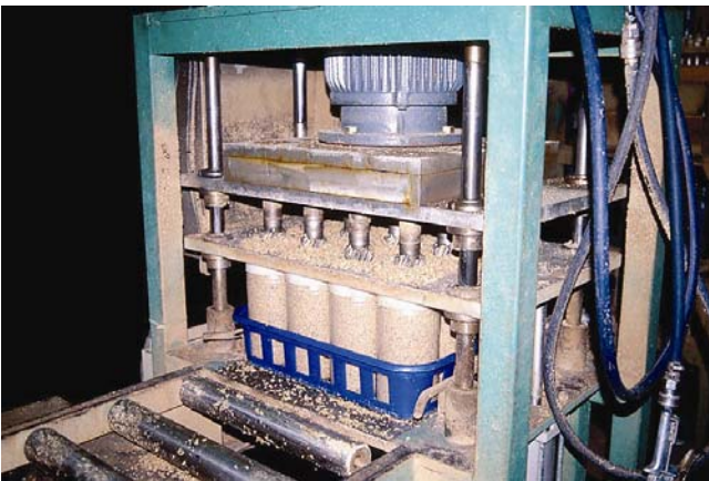
Figure 7. Feeding, compacting and hole making
