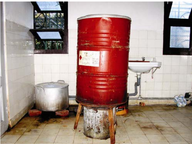
Figure 4. Drum for normal pressure sterilization
