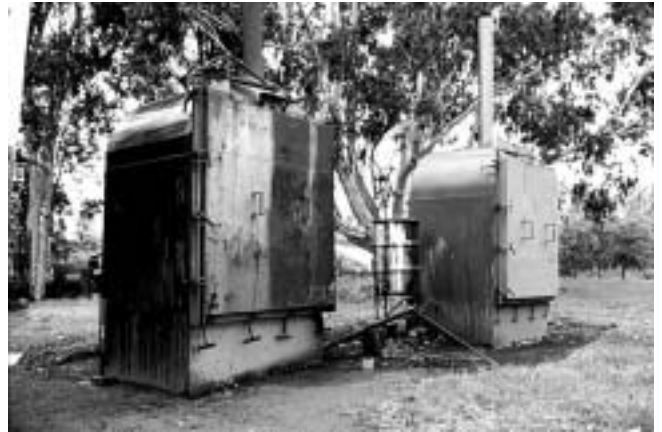
Figure 9. Locally made sterilizers for bags
