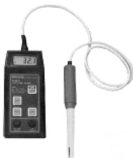
Figure 9.14 - Ppm reader (TDS meter).
