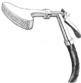
Ross watering fan attached to a variable water pressure gun
