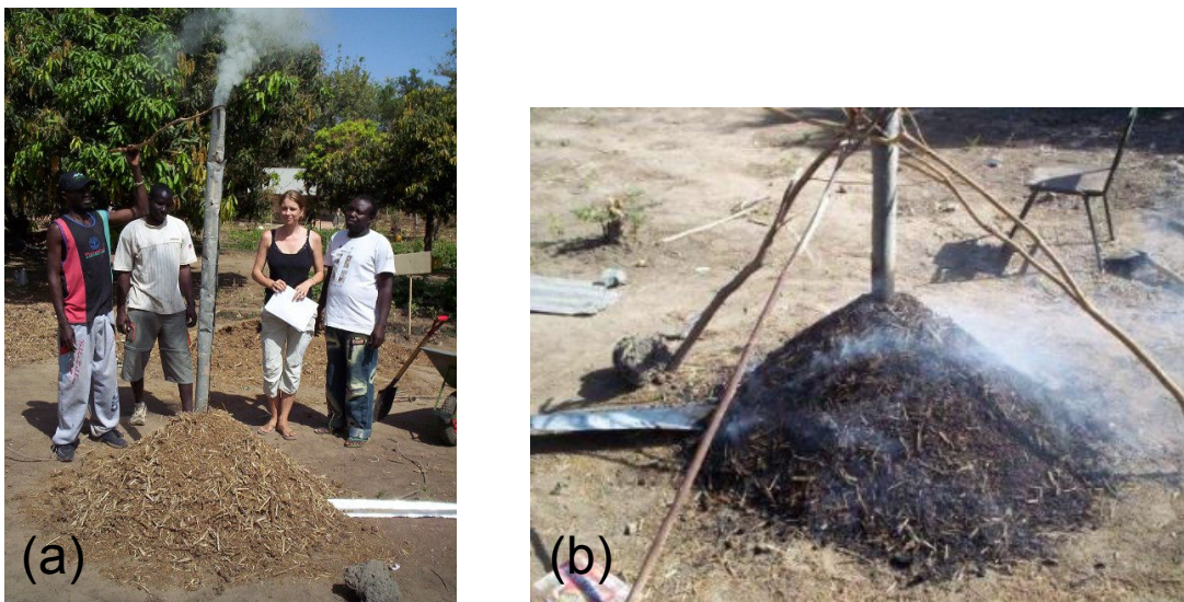
Figure 3.4: Carbonized millet husk production in the Gambia (a) and detail of the air inlet used to ensure good combustion of the millet husk mixture (b)
