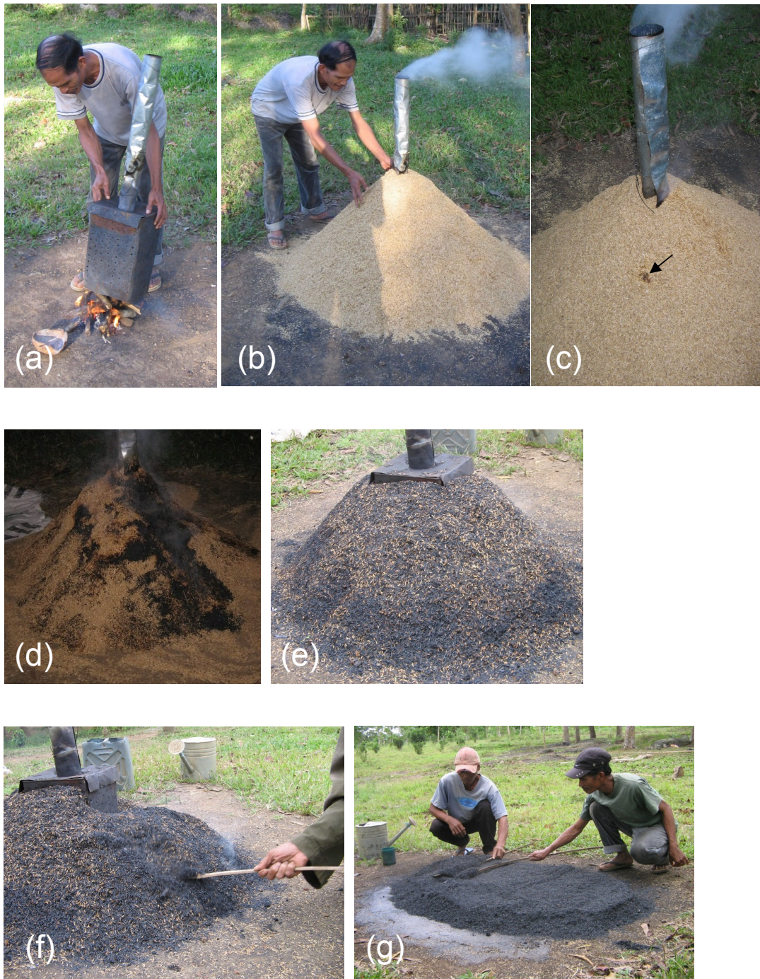
Figure 3.3: The steps of rice hull carbonization. Starting the fire and installing the carbonizer (a), adding hulls to the carbonizer (b), the appearance of carbonized areas on the rice hull pile (arrow) (c), the progression of carbonization (d), the appearance of the pile when approximately 90% of the carbonization has occurred (e), stirring the rice hulls during the final stage of carbonization (f) and spreading out the carbonized rice hulls and halting the carbonization (g).
