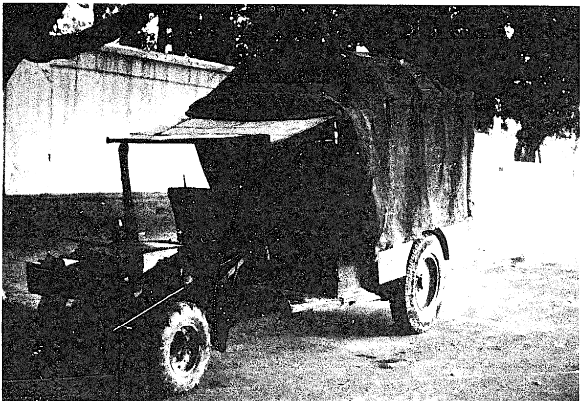
Fig. 6.2 Single-axle tractor and trailer from China. The trailer has a beam axle suspended on leaf springs, and is fitted with simple bodywork to protect the driver
