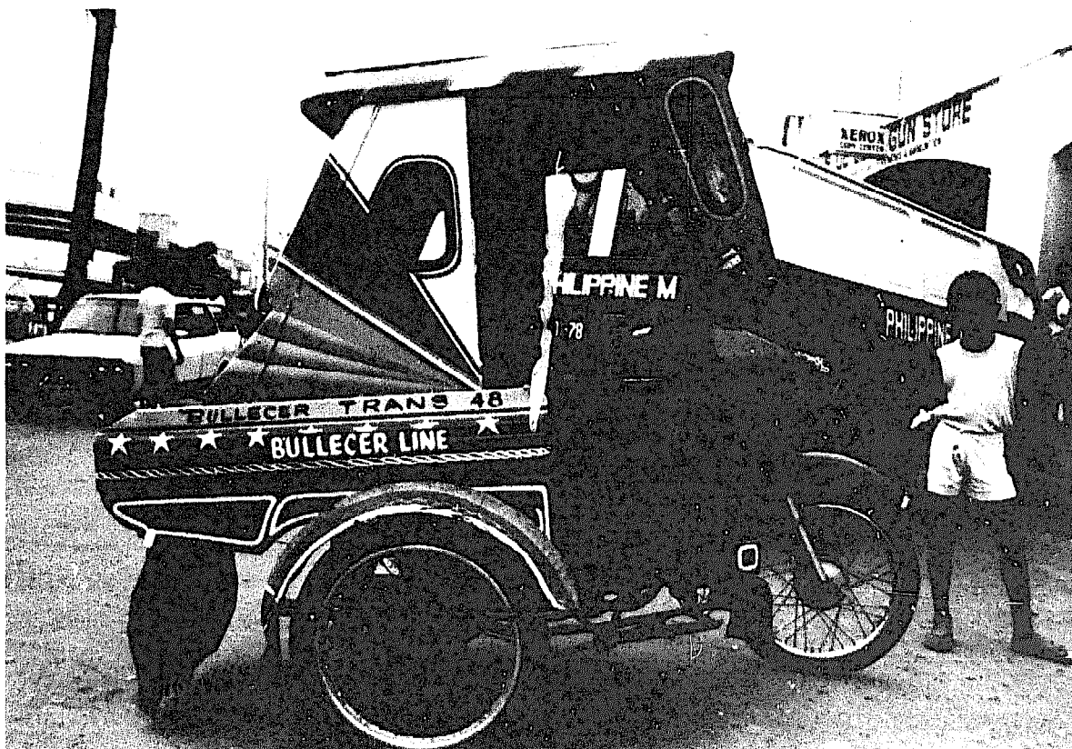
Fig. 3.22 Sidecar with combined passenger and cargo body
