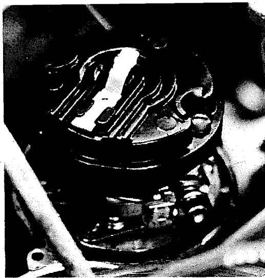
(left) GM-type rotor and distributor require slightly different service techniques than other distributors. (right) Non-GM distributor with rotor, points and condenser in place. Always note where the wires run from and connect to.
