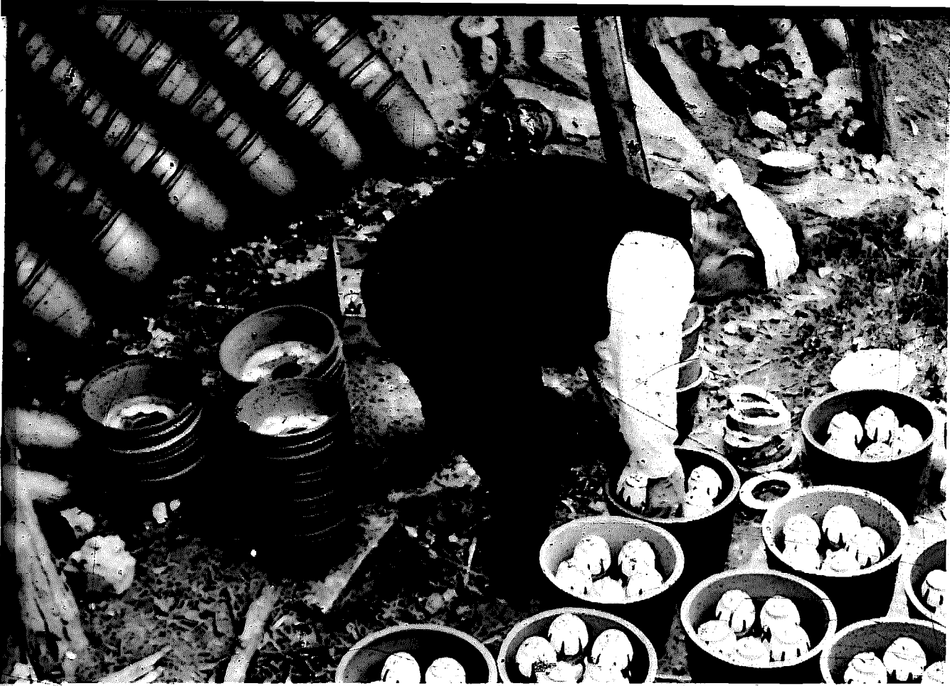
145. Unstacking a Japanese kiln. The small jars have been fired inside the larger flowerpots which serve as saggers.
