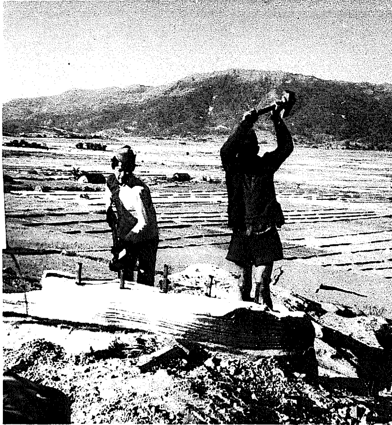
Above: Wedges are inserted into sandstone then split with sledge-hammers in Nepal.
