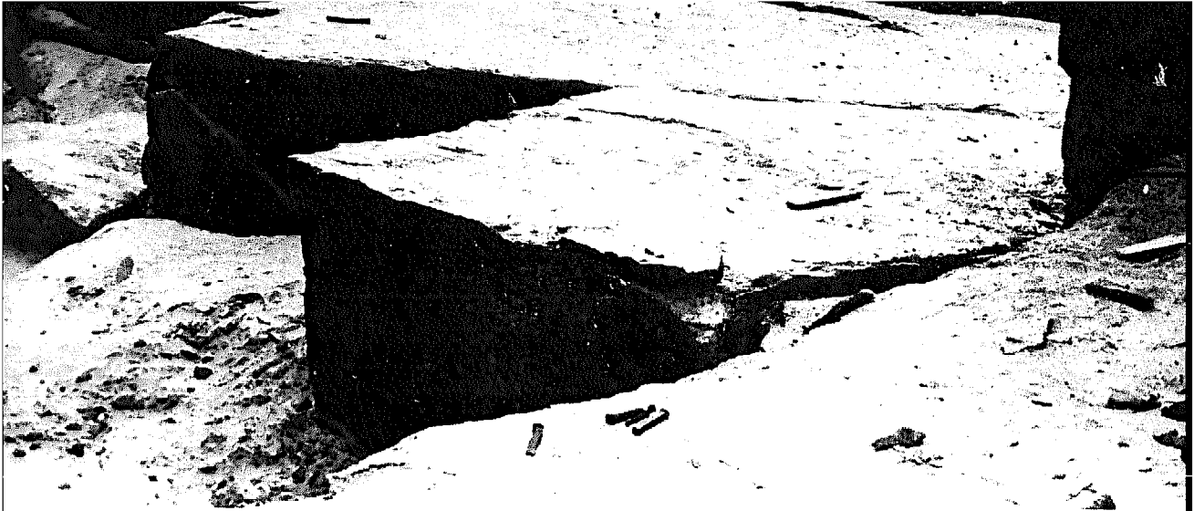
Above: The well-spaced jointing of this granite quarry facilitates the removal of industrial-sized blocks. Below: Another example of widely spaced jointing, this time in a hillside deposit of well-bedded marble.
