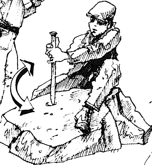
Drilling holes in a large block with a hand drill before breaking with plugs and feathers
