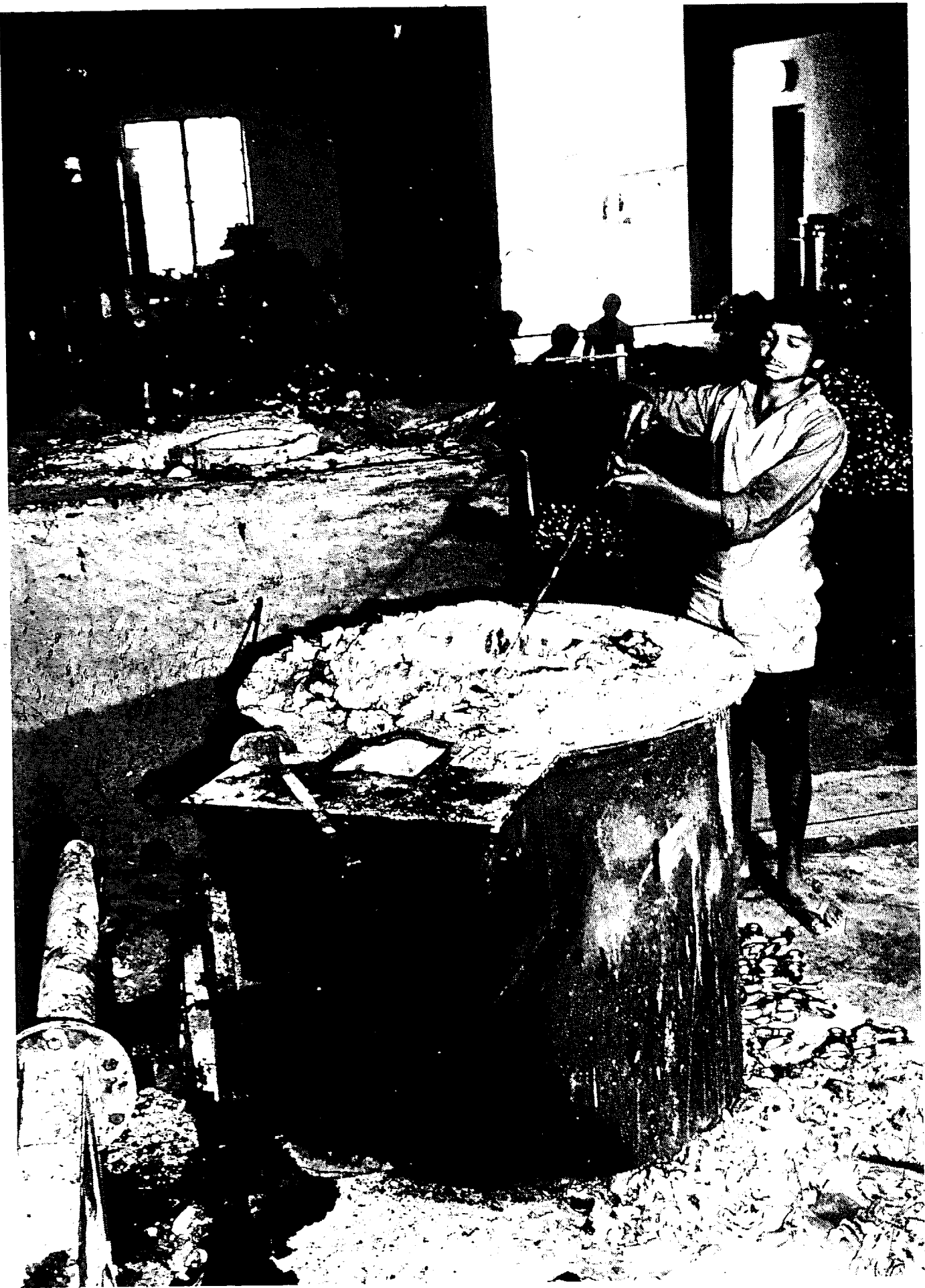
Precision Foundry - the oil-fired furnace for melting aluminum; the coal-fired furnace, used when power fails, is behind.
