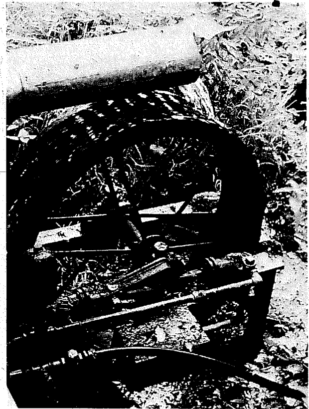
Fig 2.61 A small overshot waterwheel driving reciprocating pumps at Nantellan, near Grampond, Cornwall
