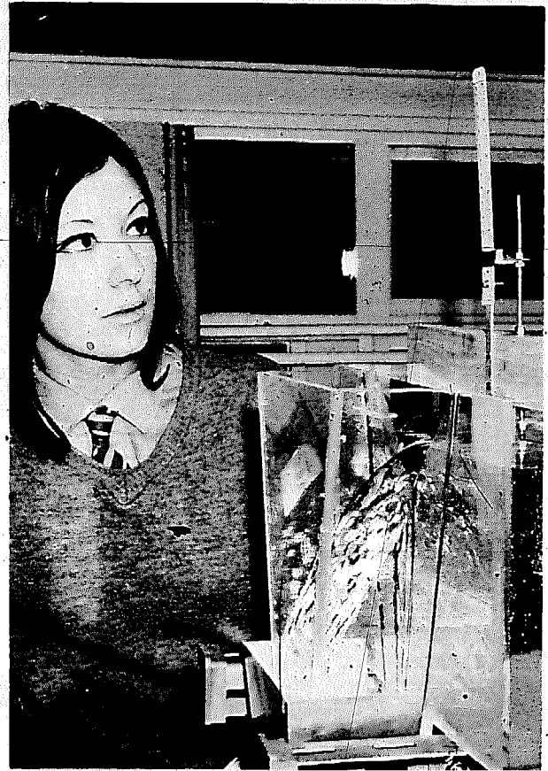
2.28 A pupil from the Dunsmore School for Girls, Rugby, observing the head of water flowing over a V-notch. Note that the sides of the notch are chamfered to present a sharp edge. The scale is fixed to the cross member but the screwed rod, carrying the pointer, is adjustable so that its lower end, pointed and bent through 180° to point upwards, just touches the surface of the water about 75 mm upstream of the notch
