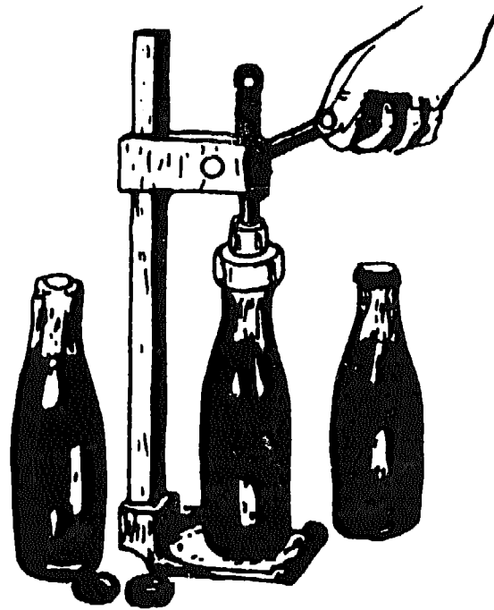
figure 10: A metal bottle top sealer
