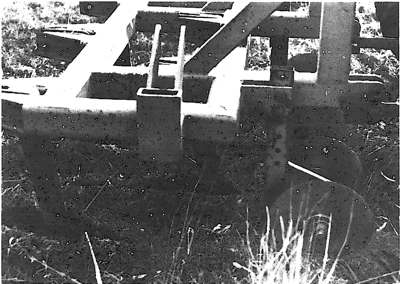
PLATE 3.2 : DETAIL OF WALLACE SOIL CONDITIONER. COULTER SPLITS SOIL, HAPTED 'SHOES' FOLLOW, TO MAKE AIR TUNNELS BELOW SOD.
