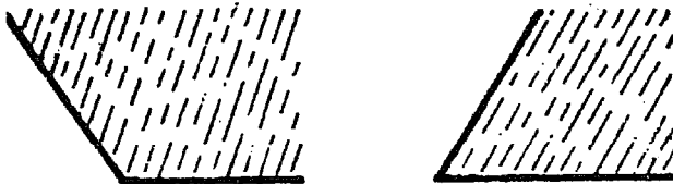
These two corners are not square. They do not make right angles.
