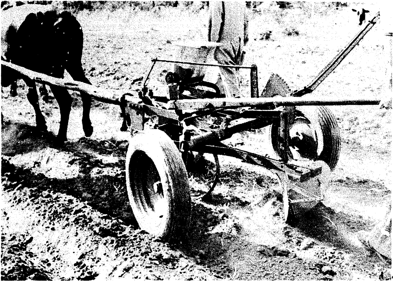
Fig. 5-14: Wheeled toolcarrier based on old front axles of a tractor, Zambia, 1985. (Photo: J. Rauch).
