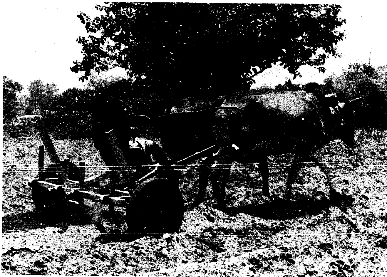
Fig. 4-19: NIAE wheeled toolcarrier being used for ridging in Yemen, 1973. (Photo: AFRC-Engineering archives).
