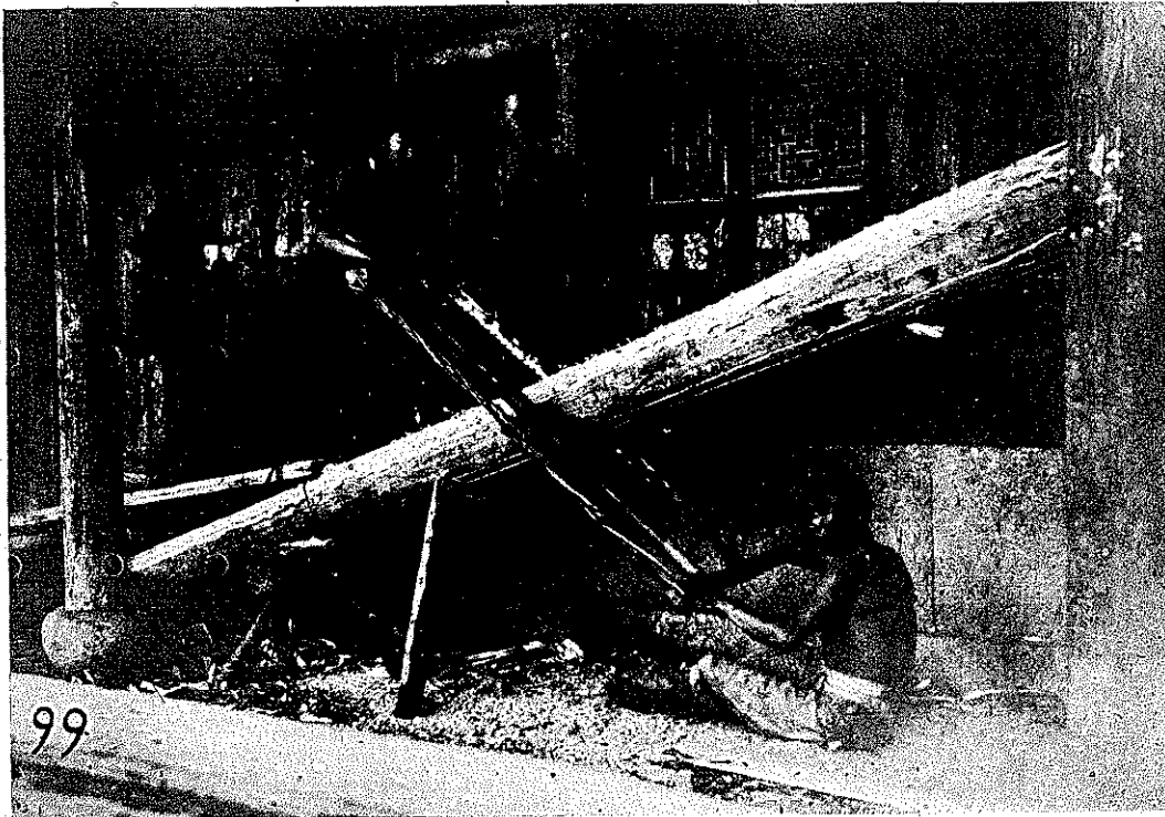
FIG. 327. CHINESE BOARD SAWYERS, SAWING A LOG INTO BOARDS.
