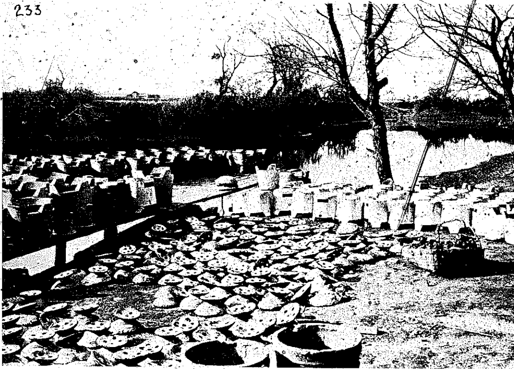
FIG. 206. DRYING CHARCOAL STOVES.
