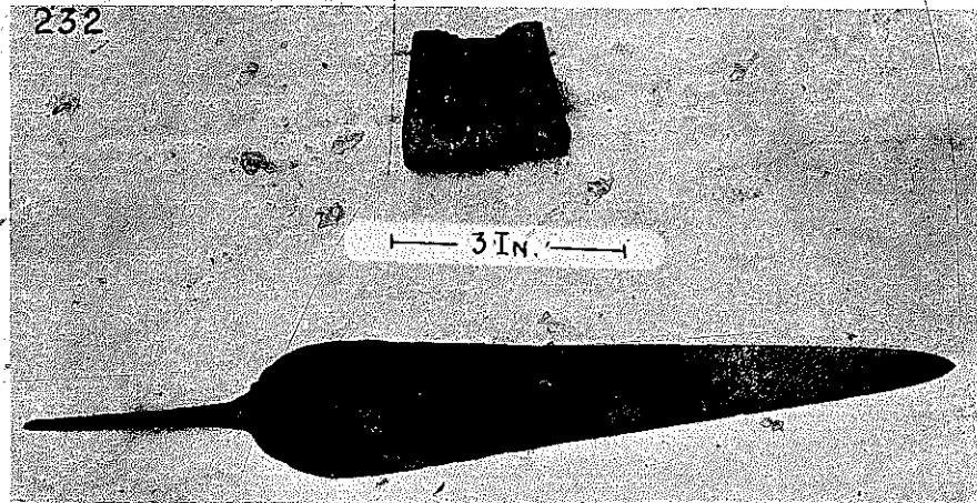
FIG. 205. STOVE MAKER'S CLAY KNIFE (LOWER) AND CHOP OR TRADEMARK CLAY STAMP (UPPER).
