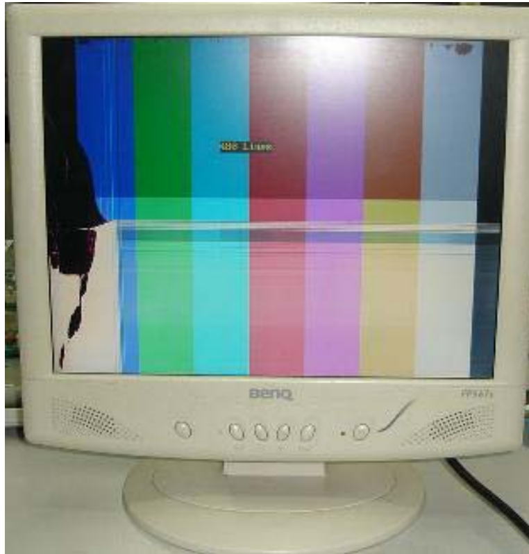
A cracked panel in BenQ 15" LCD Monitor
