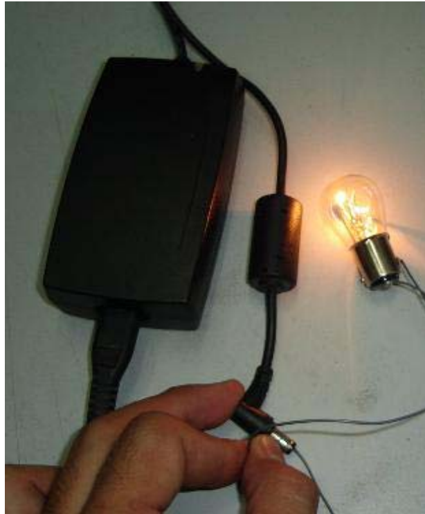
Using automobile light bulb to test the regulation of the power adapter
