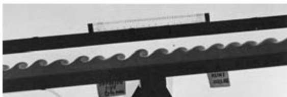
Fig. 4.48 Kelvin–Helmholtz waves formed at a sharp, shearing interface between clear up-tank moving less dense fluid and dark down-tank moving denser fluid. Note shape of waves, asymmetric upflow. Pressure deviations from Bernoulli accelerations amplify any initial disturbances into regular vortices.
