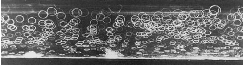
Fig. 4.44 Time-lapse photograph of shallow water wave orbitals visualized by tracer particle. This flow visualization of suspended particles was photographed under a shallow water wave traversing one wavelength, \lambda , left to right. Wave amplitude is 0.04\lambda and water depth is 0.22\lambda . The clockwise orbits are ellipses having increasing elongation toward the bottom. Some surface loops show slow near-surface drift to the right. This is called Stokes drift and is due to the upper parts of orbitals having a greater velocity than the lower parts and to bottom friction. The surface drift is accompanied by compensatory near-bed drift to the left, due to conservation of volume in the closed system of the experimental wave tank. Stokes drift without the added effects of bottom friction also occurs in short, deep water waves.
