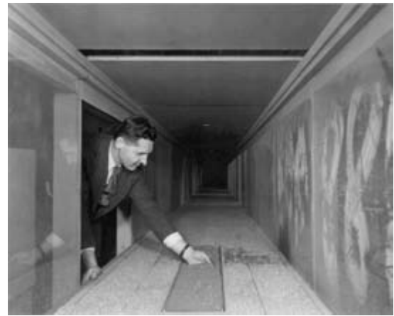
Fig. 4.36 (left) W.S. Chepil made the quantitative measurements of lift and drag used as a basis for Fig. 4.35. Here he is pictured adjusting the test section of his wind tunnel in the 1950s. Much research into wind blown transport in the United States was stimulated by the Midwest “dust bowl” experiences of the 1930s.
