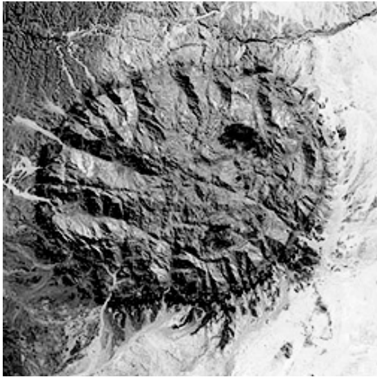
Fig. 5.20 The surface trace of an igneous pluton as seen from space. This is the granitic Branberg Massif, Namibia, elevation 2.5 km. The near-circular outcrop can be taken to represent a horizontal slice through the crust. Pluton long axis is 30 km. The slightly darker outer rim is the marginal zone of contact between the intrusive granite and ambient sedimentary strata into which the pluton intruded.
