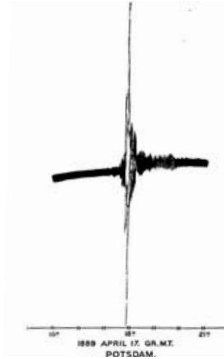
Fig. 4.129 An historic seismic record: facsimile of the 1889 Tokyo earthquake recorded by Paschwitz at Potsdam, Germany.
