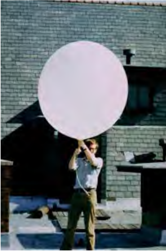
A radiosonde weather balloon being prepared for launch. Such balloons measure wind, temperature, and humidity to heights above 100,000 feet.
