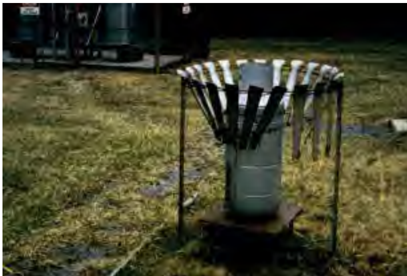
A rain gauge with a wind screen used to lessen the amount of catch (rain) missed due to rain streaming over the edge of the gauge. FMA, INC.
