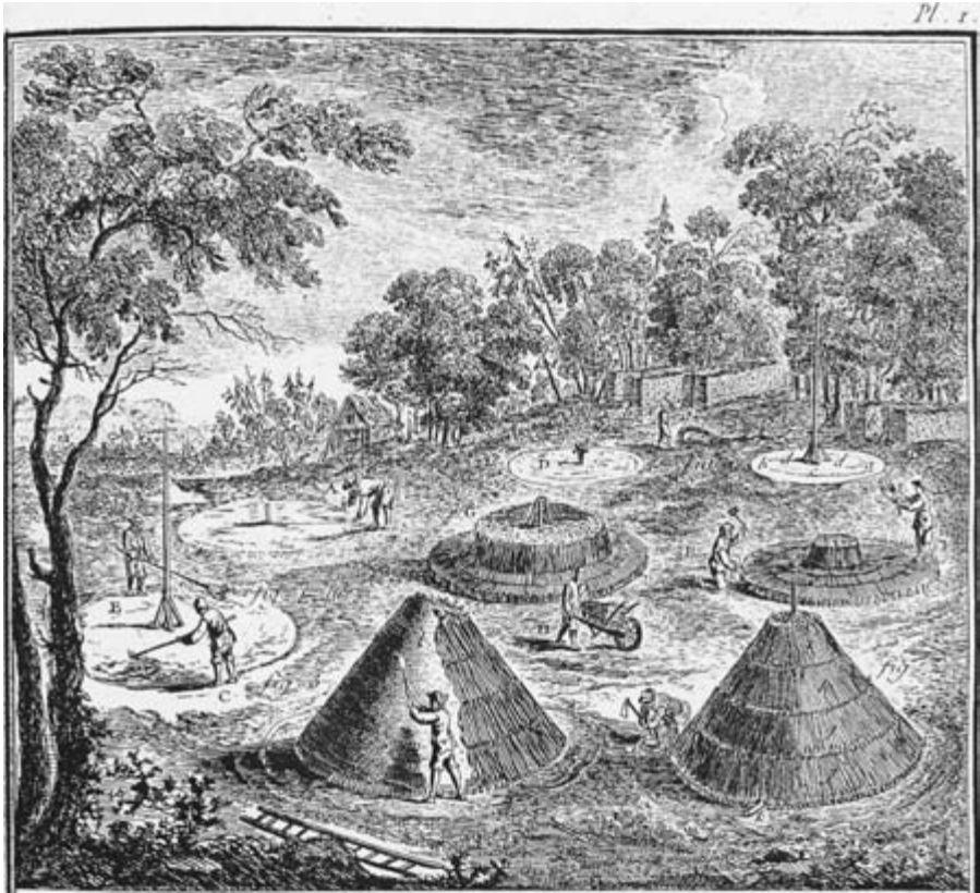
Plate 7.2 Preparing and making charcoal. Woodcutters brought the wood to the kiln area, where the charcoal producers stacked it methodically in cone or beehive form and then covered all with a coating of clay or earth (I, this page). This kept the inner temperature at a minimum, so that the wood smoldered and was eventually converted to charcoal and not ash. After the cone was lit (II, 169, right foreground), the pile was progressively reduced in size until pure charcoal remained. (From D. Diderot, Encyclopedie . . . Recueil de planches sur les sciences, les arts liberaux, et les arts mécaniques [Paris, 1763], vol. 1.)
