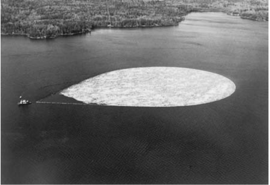
Plate 9.2 Sometimes the products of the individual log drives could be collected within a towable boom. In this view the boom is being towed by steam tug across Rainy Lake, Ontario, to the mill of the Minnesota and Ontario Paper Company at Fort Frances. (Forest History Society, Durham, N.C.)
