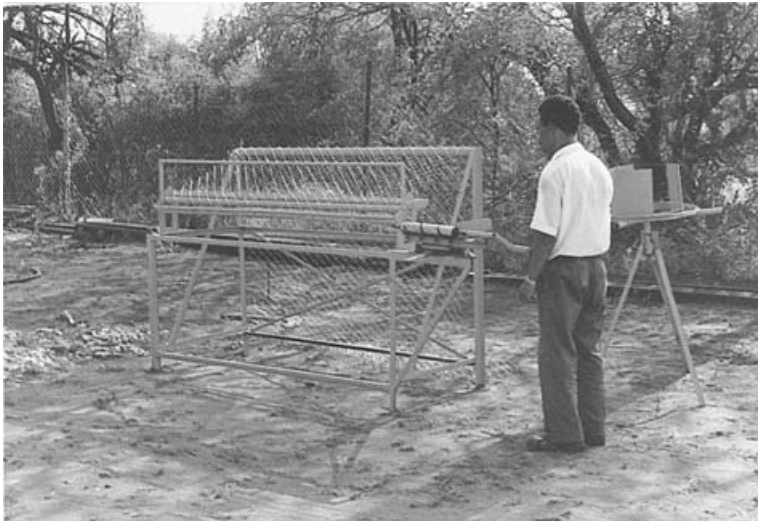
FIGURE 26 Wire fencing making machine made at RIIC in Botswana. (From RIIC Catalogue of Goods and Services , 3rd Edition.)
