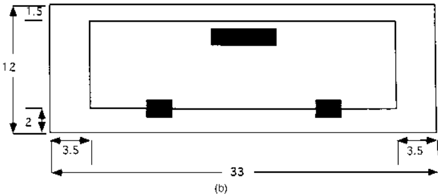
FIGURE 48b Front with door, handle, and hinges The door is fixed to the front part and attached with hinges (shown). A handle (dark bar) made of scrap wood is also attached (glue and, if needed, two nails).
