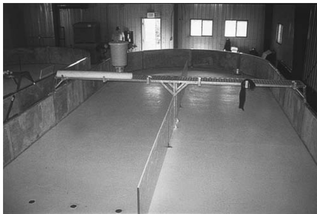
Figure 10. Recirculation system growout tank for summer flounder.
