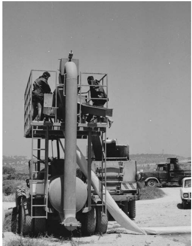
Figure 2. A large fish pump (Israel). The fish are sorted by workers who separate them into marketable and submarketable groups. Submarketable fish are returned to a pond for further growout.
