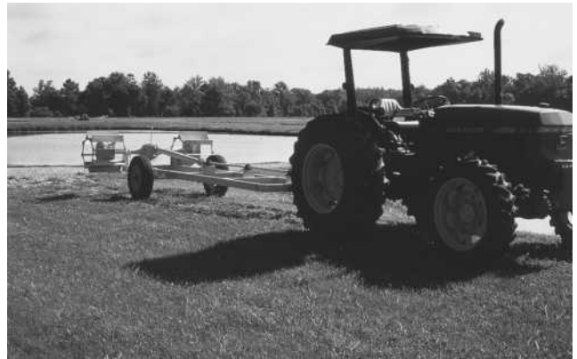
Figure 3. Paddlewheel aerator powered by the PTO of a tractor.
