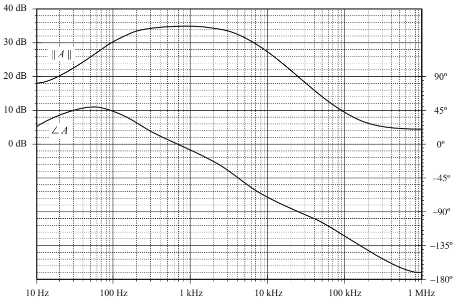
Fig. 8.66 Experimentally measured magnitude and phase data, Problem 8.5
