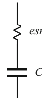
Fig. 20.12 Capacitor equivalent circuit. Losses are modeled by an equivalent series resistance (ESR)
