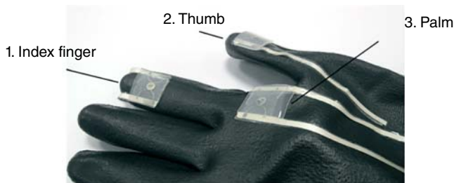
Figure 9.14 Positions of the sensors: index finger, thumb, and palm region. Source: Yeo et al. 2016 [25]. Copyright 2016, Reproduced with permission of Royal Society of Chemistry.
