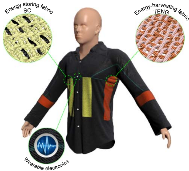
Figure 4.9 The scheme of a self-charging power textile that integrates energy-harvesting, energy storage, and functional electronics. Source: Pu et al. 2016 [29]. Copyright 2016, Reproduced with permission of John Wiley and Sons.
