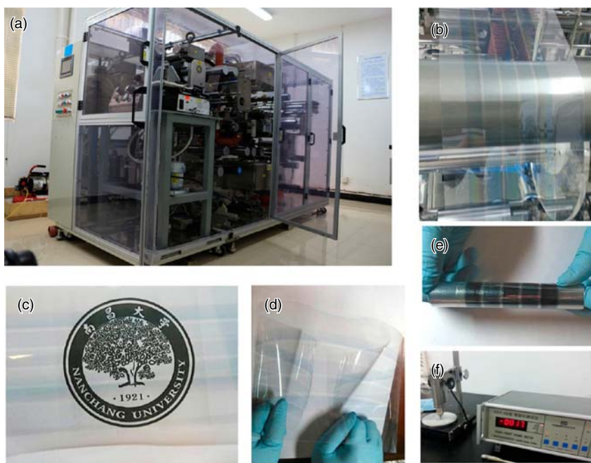
Figure 5.10 (a) Roll-to-roll machine, (b) roll-to-roll process of PEDOT:PSS:CNTs printing, the wet PEDOT:PSS:CNTs film (dark blue), (c–e) picture of the gravure-printed PEDOT:PSS:CNTs electrode with superior flexibility and high transparency, the corresponding dried films (light blue), and (f) transparent PEDOT:PSS:CNTs electrode coated onto PET substrate showing the best sheet resistance of 17 ( \Omega/\text{sq} ). Source: Hu et al. 2014 [35]. Copyright 2014, Reprinted with permission of American Chemical Society.
