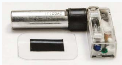
The revolutionary new capacitor material is the flat black object below the aluminium xenon flash tube holder
