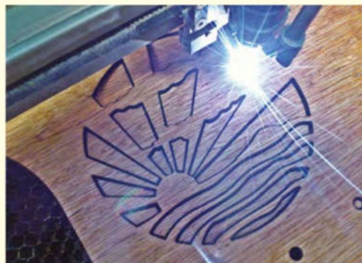
Fig.17. Laser cutting the retro-design radio enclosure
