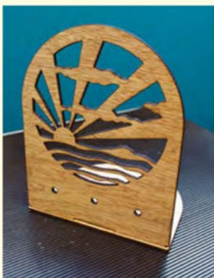
Fig.18. Assembled case parts awaiting the electronics fit
