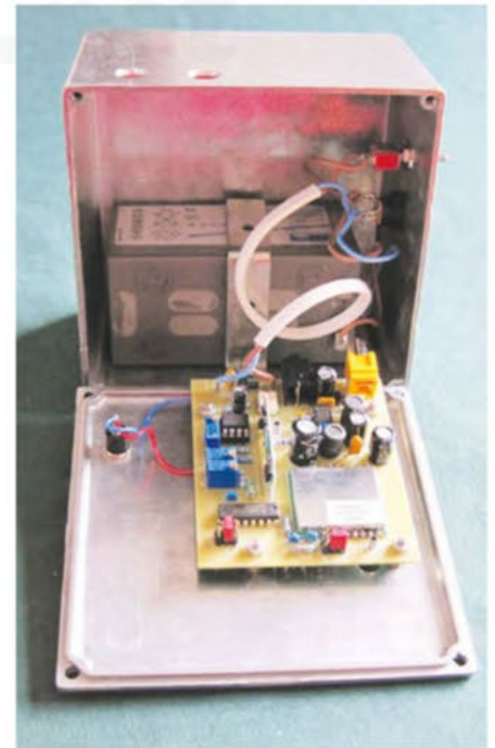
Fig.6. The battery-powered transmitter
