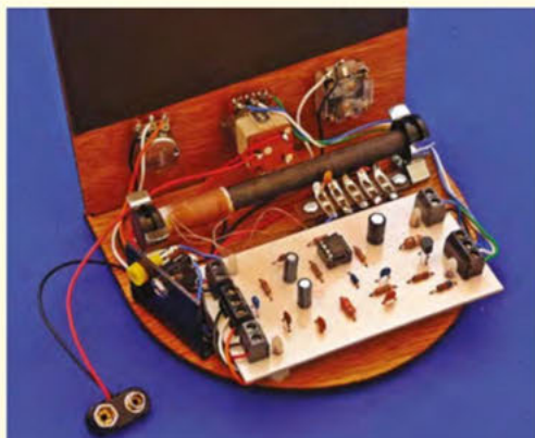
Fig.19. Rear view of radio showing our component layout
