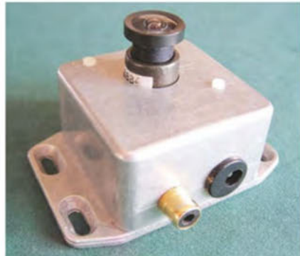
Fig.2. The diecast box sealed ready to be put in position
