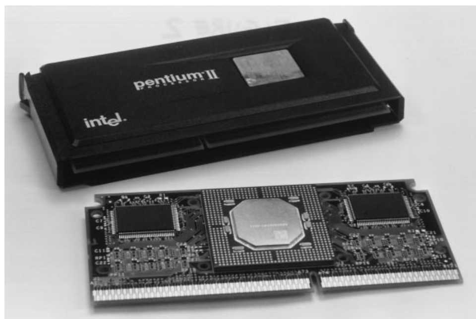
Figure 2. The 1998 successors to the line of microprocessors started by the 4004, Intel's Pentium II processor, mounted within its Single-Edge Cartridge Connector (SECC). This picture shows the cartridge with its black case removed. On the substrate within the cartridge, the large octagonal package in the center is the Pentium II CPU itself. The rectangular packages to the right and left of the CPU are the cache chips. The small components mounted on the substrate are resistors and capacitors needed for power filtering and bus termination.
