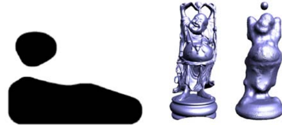
Figure 20. The stability map (top left) indicates the maximum radius of a ball that can reach the point without intersecting the shape. Tightening fills in cracks and removes constrictions and small components (top right and bottom left). Tightening of a 3-D shape (bottom right).
