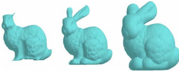
Figure 18. The original shape (center), its grown version, (right) or shrunk version (left) (137).
