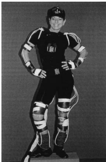
Figure 5. A performer wearing a motion capture apparatus. The device shown is a full body magnetic tracking system. Image courtesy of Robert E. Bodenheimer, Jr.
