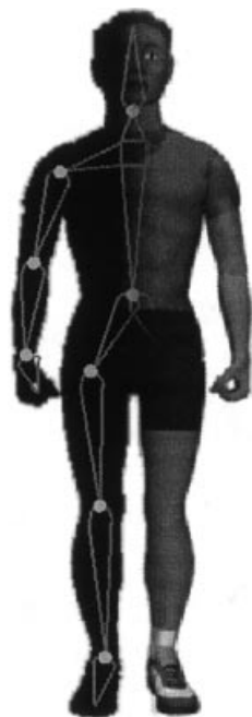
Figure 2. An articulated model of a human male. The structure of the joint hierarchy is shown on the left. The graphical model used for rendering is shown on the right. Image courtesy of the Graphics, Visualization and Usability Center, Georgia Institute of Technology.
