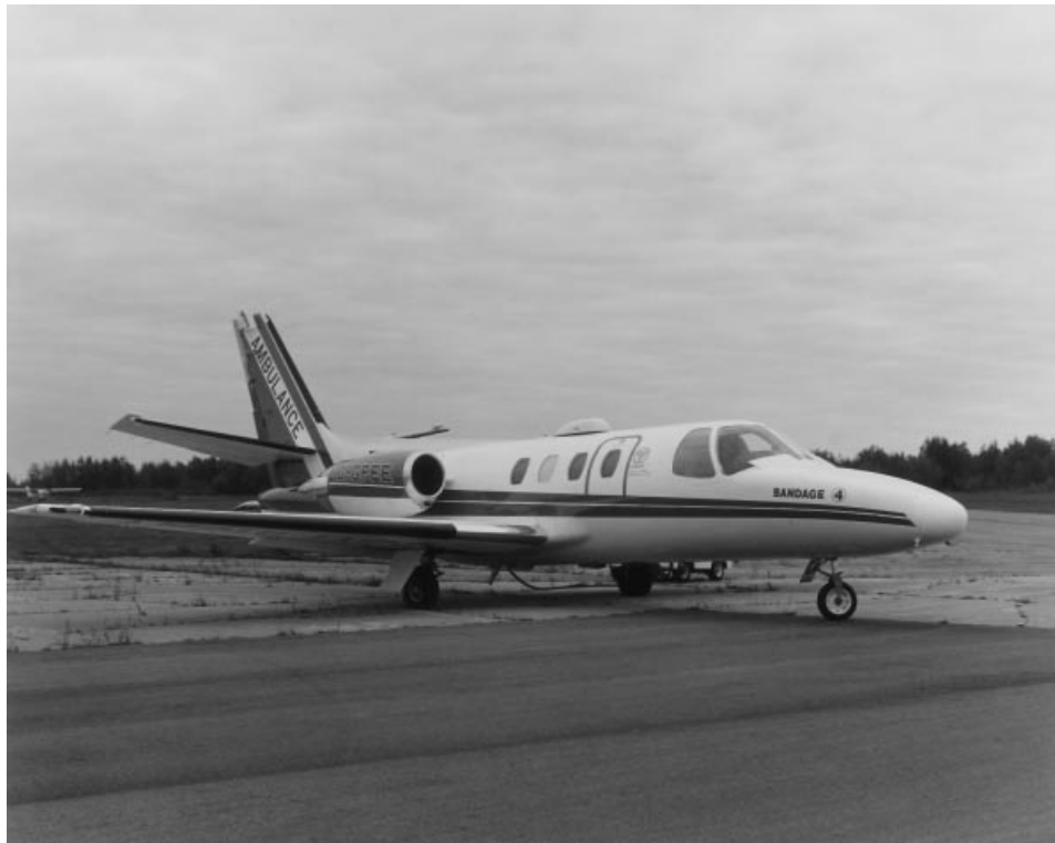
Figure 6. A Cessna Citation jet aircraft, operated by the Ontario Air Ambulance Service, equipped with a mobile satellite communications terminal. The antenna subsystem can be seen mounted on the top of the fuselage.
