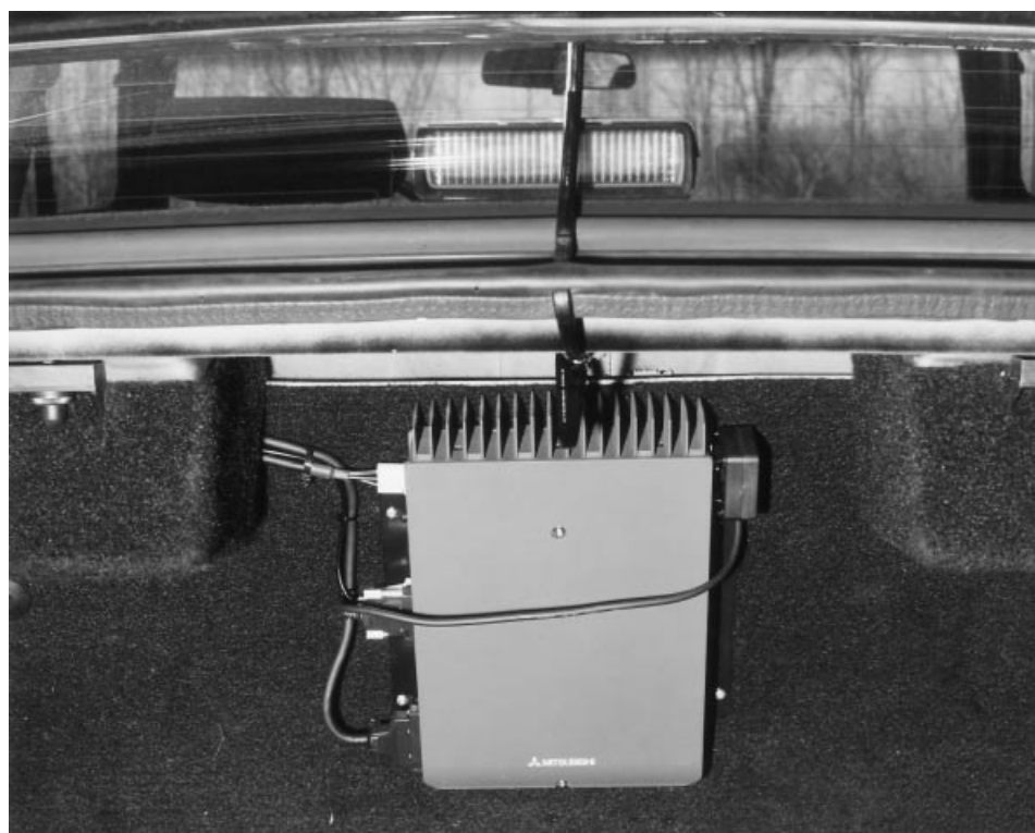
Figure 3. A Mitsubishi MSAT telephone transceiver mounted on the front wall of the trunk of a car.
