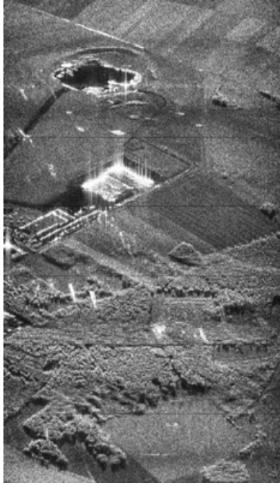
Fig. 14. An example of an ESAR-2 strip-map SAR image. It is processed by the range-migration algorithm. The ESAR-2 data are made available by courtesy of the German Aerospace Research Establishment (DLR).
