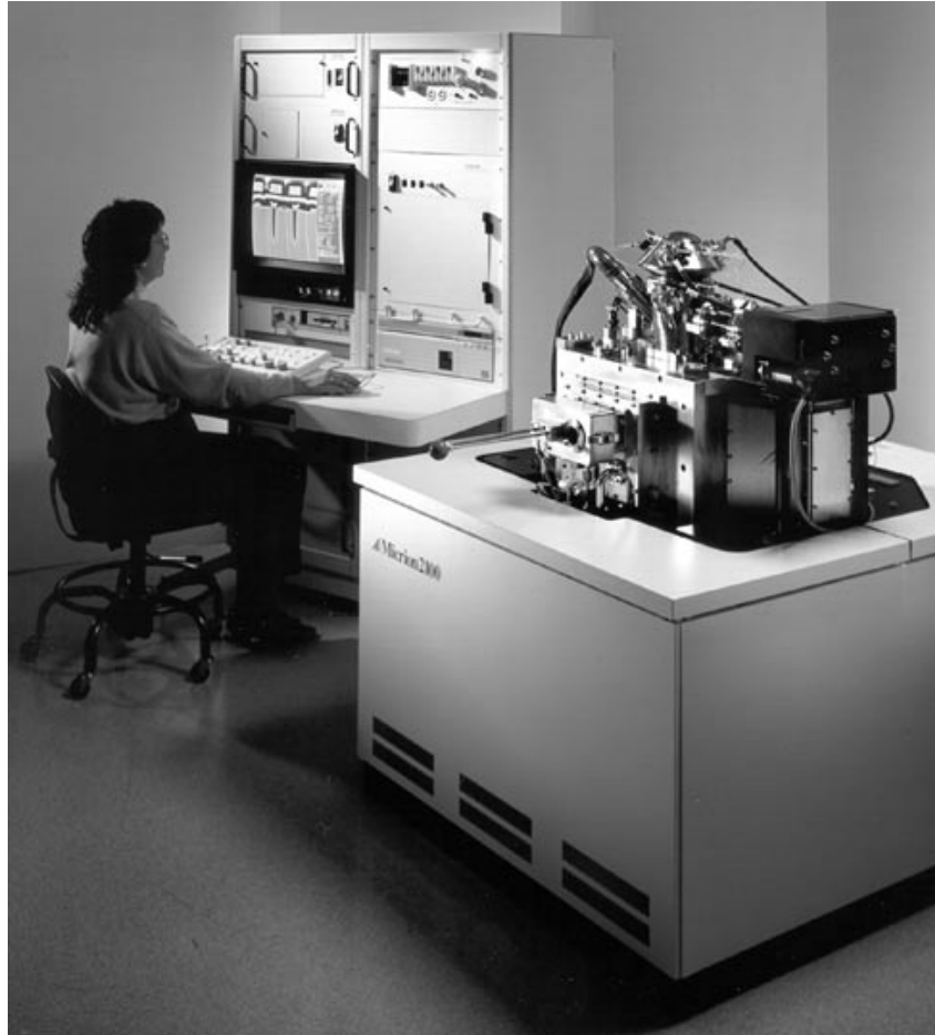
Fig. 4. A photograph of a focused ion-beam system showing the ion column mounted on a vacuum chamber.
