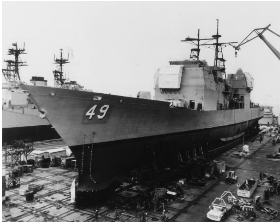
Figure 5. A spherical, midfrequency sonar array on the bow of a cruiser in drydock.
