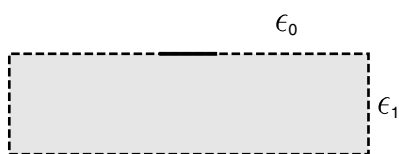
Figure 2. Cross section of a microstrip line.
