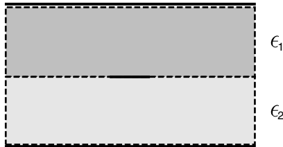
Figure 1. Cross section of a stripline.
