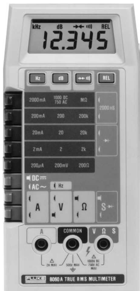
Figure 14. Photograph of the Fluke 8060A true rms multimeter. Reproduced with Permission from Fluke Corporation.
