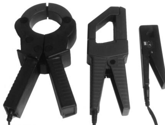
Figure 15. Example of a clamp on DMM. Photo by Bill Dabbs.
