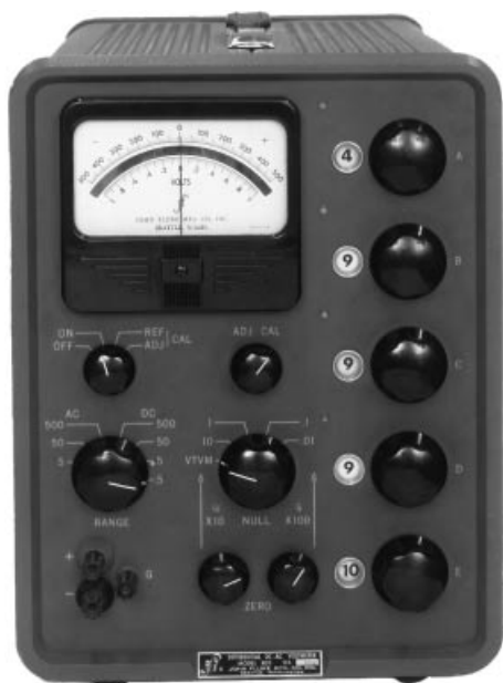
Figure 7. Photograph of the Fluke 803 differential dc-ac voltmeter. Reproduced with permission from Fluke Corporation.
