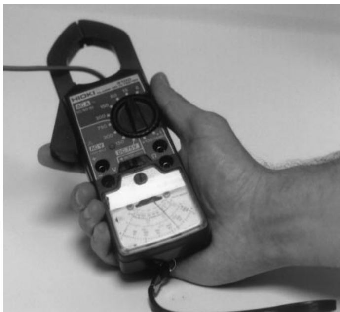
Figure 16. Example of common current probes available for use with DMMs. Photo by Bill Dabbs.
