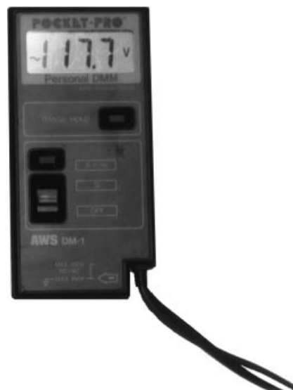
Figure 10. Example of a typical pocket DMM. Photo by Bill Dabbs.
