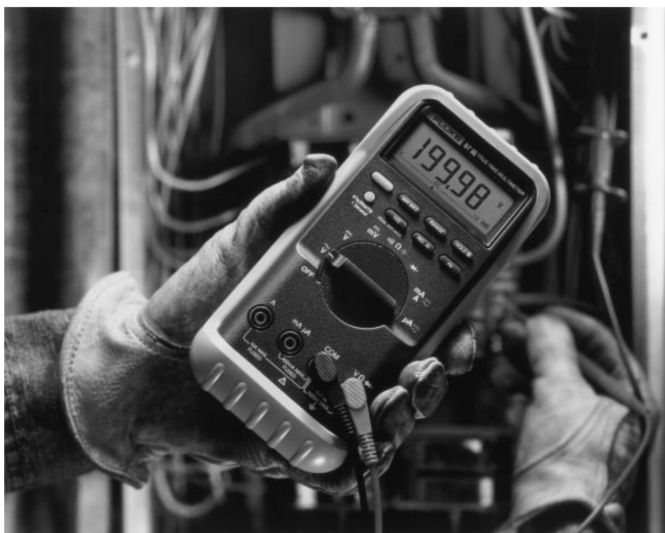
Figure 13. Photograph of the Fluke 87 III true rms multimeter. Reproduced with Permission from Fluke Corporation.
