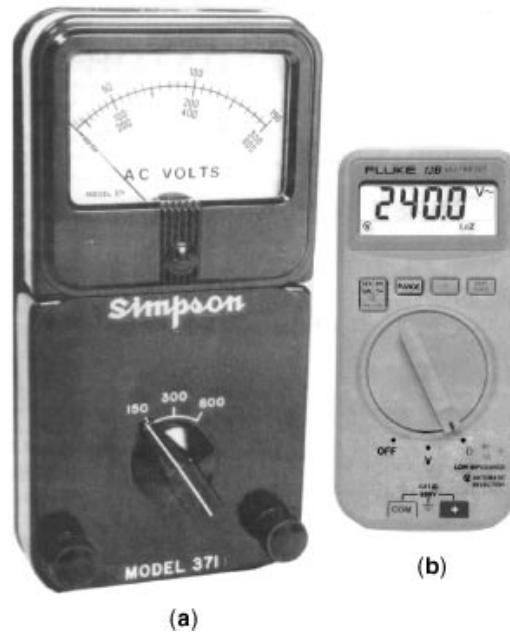
Fig. 1. (a) Analog voltmeter, simpson model 371 (courtesy of Simpson). (b) Digital voltmeter, Fluke model 12B (courtesy of Fluke).
