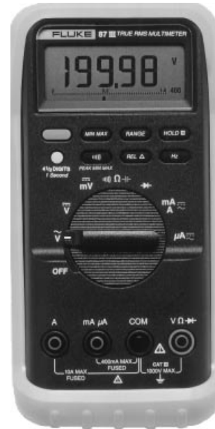
Figure 1. Modern full feature DMM (Fluke 87 III).
