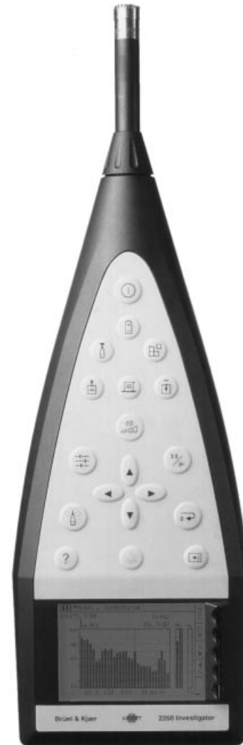
Figure 4. An example of the basic instrument for acoustical measurements, a sound level meter (courtesy of Brüel & Kjær Instruments, Inc.).
