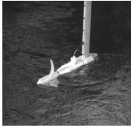
Fig. 5. Rotating-element current meter with horizontal axis nearly parallel to the direction of flow. The local flow velocity is proportional to the angular velocity of meter rotor.
