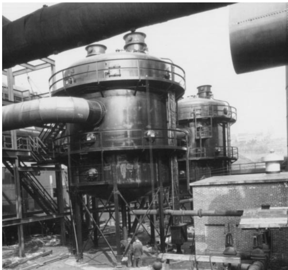
Figure 2. Two wire-tube precipitators. The gas enters at the bottom (not visible), flows up through individual small diameter tubes, and out the top sides. Electrical power to the corona wires is supplied from the two cylindrical metal enclosures on top of each unit. Collected liquid particles flow down through the tubes to drop into a hopper and drain below each unit. (Photograph courtesy Research-Cottrell, Inc., Somerville, NJ © 1997 by Research-Cottrell. All rights reserved.)
