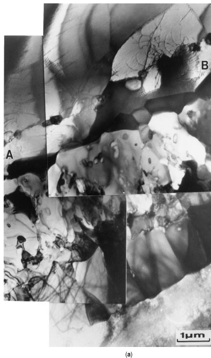
Figure 10. Transmission electron micrograph of the intermetallics at the interface of the couple AISI/316L/Ti6242 diffusion bonded (44).
