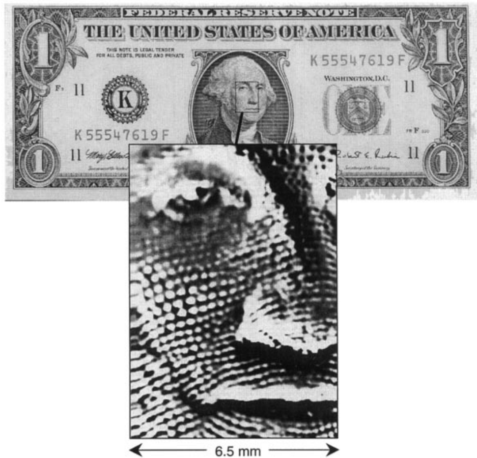
Figure 4. Inset shows the magnetic image of a portion of George Washington's face on a $1 bill observed with an HTS SQUID microscope. Data provided courtesy of T. S. Lee, G. Dantsker, and J. Clarke University of California, Berkeley.
