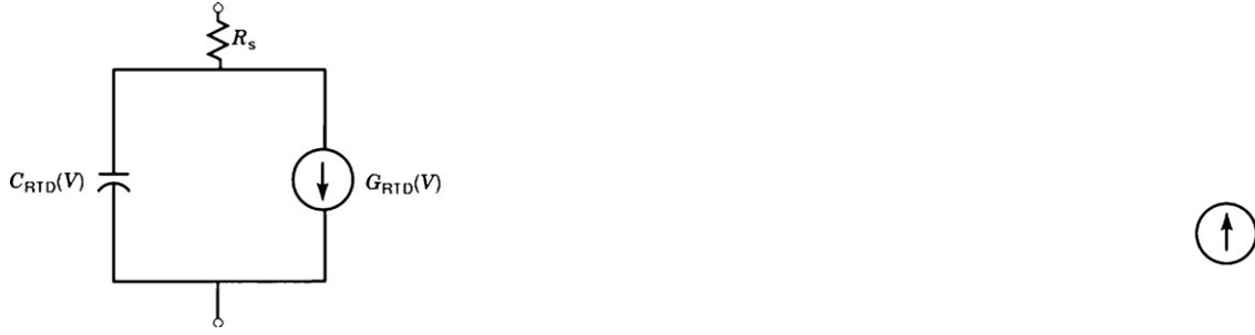
Figure 5. Equivalent circuit of the RTD. This circuit consists of a voltage-dependent current source, a voltage-dependent capacitor, and a series resistor.
