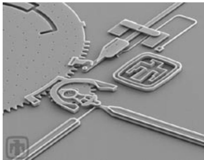
Figure 5. A scanning electron micrograph of a complex surface micromachined mechanism. The mechanism in the center converts the linear motion of the long beam on the right to a rotary motion of the small gear. Note that two different structural polysilicon layers are used. (Courtesy of Sandia National Labs.)
