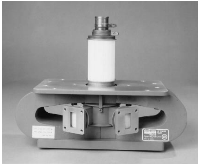
Figure 12. Photograph of an X-band backward wave CFA.
